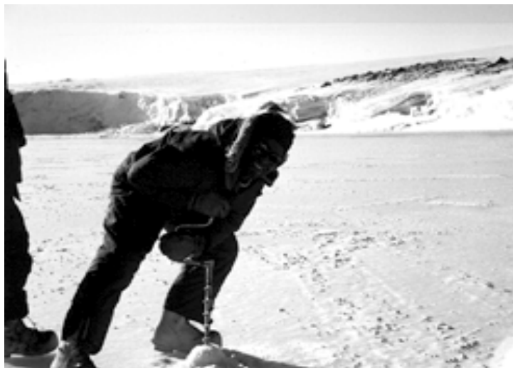
Figure 17-8: Drilling ice with Kovacs Ice Auger. (photo by Tim Cully)
